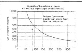
Measure the gas concentration level in the environment and plot it on the Y-axis on the breakthrough curve. Draw an extension line from that point, parallel to the X-axis towards the breakthrough curve. The estimated service life is the value on the X-axis where the extension line meets the curve.
